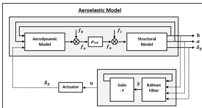
Figure 7 The block diagram of the aeroservoelastic model
