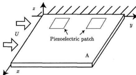
Figure 8 Plate wing with piezoelectric patches
