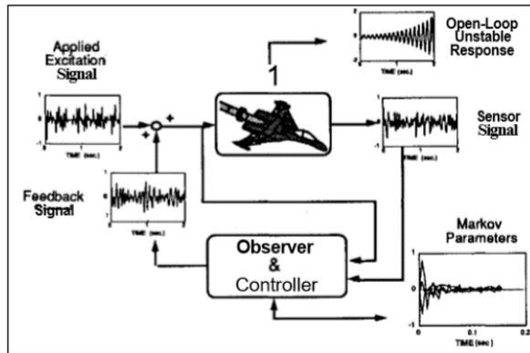
Figure 6 Identified control system from experimental data
