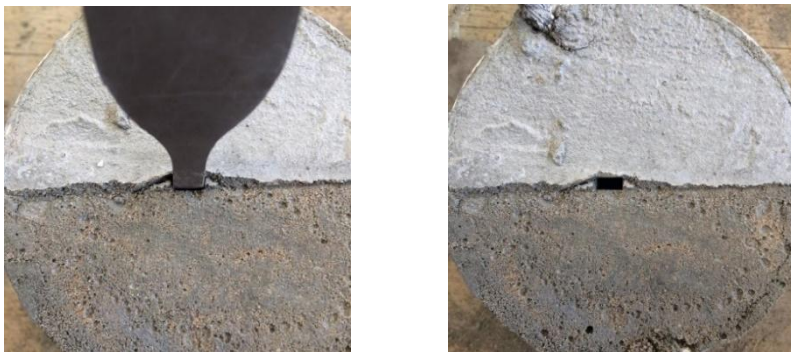
Figure 12 Concrete shrinkage from the surface of bonded rubber with fly ash as a filler
