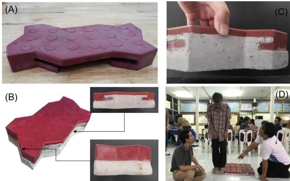
Figure 14 (A) Shock-absorbing rubber [1] (B) Paving blocks (C) Pulling adhesion test (D) Paving blocks test
