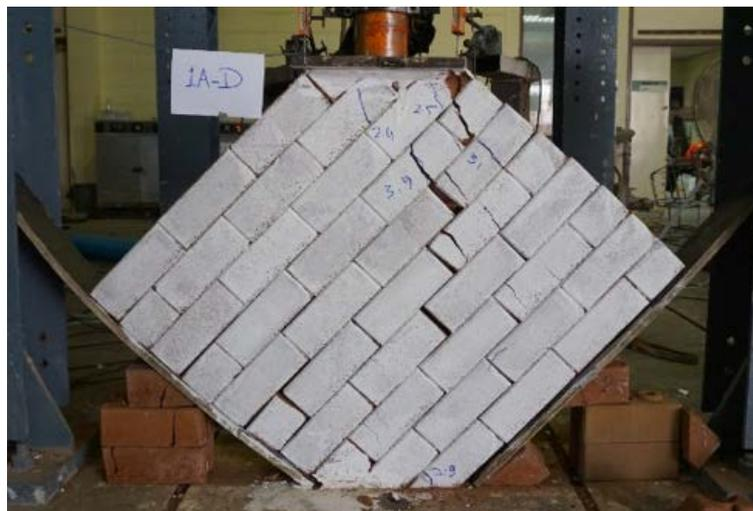
Figure 16 Failure mode of wall specimen 1-D
