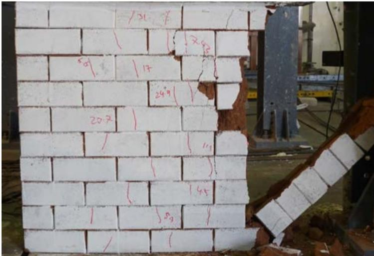
Figure 13 Failure mode of wall specimen 1-A
