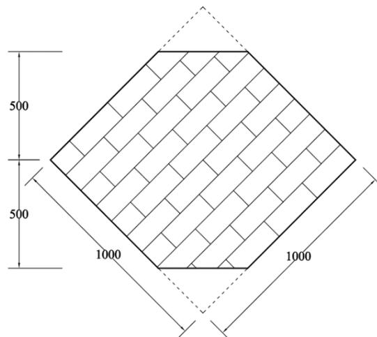
**Figure 4 Details of diagonal wall (units in mm)**
