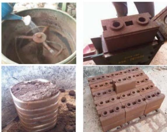
**Figure 1 Manufacturing process of interlocking hollow bricks**
