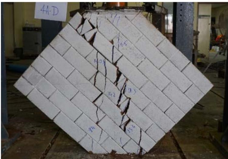
**Figure 18 Typical failure mode of cement grouted reinforced walls (Diagonal compression)**
