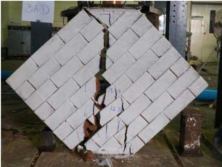
**Figure 17 Typical failure mode of cement grouted un-reinforced walls (Diagonal compression)**
