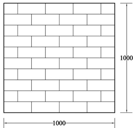
**Figure 3 Details of axial wall (units in mm)**
