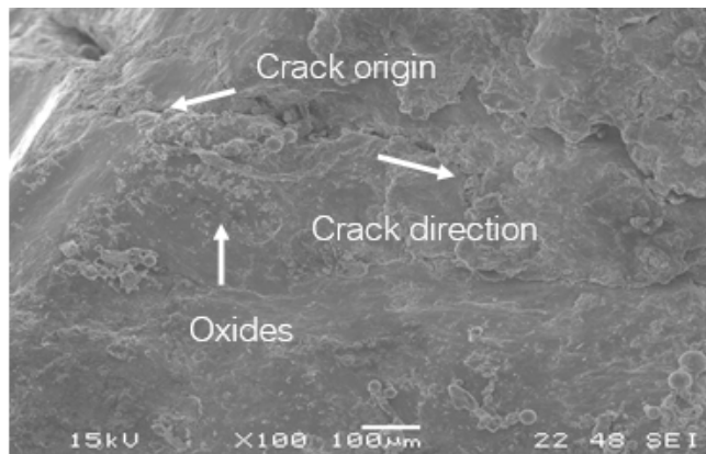
Figure 8 Fractography showing view of the crack origin and oxides
